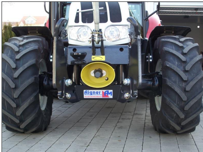
Lower links fold inward diagonally
