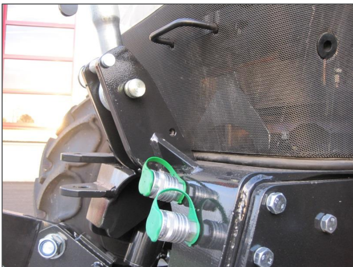
Holder for top link – integrated hydraulic connections (3 rd service kit)
