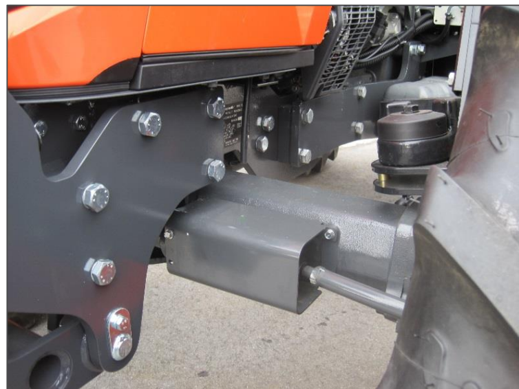
Stable frame up to clutch housing – Absolute front axle oscillation and steering angle
