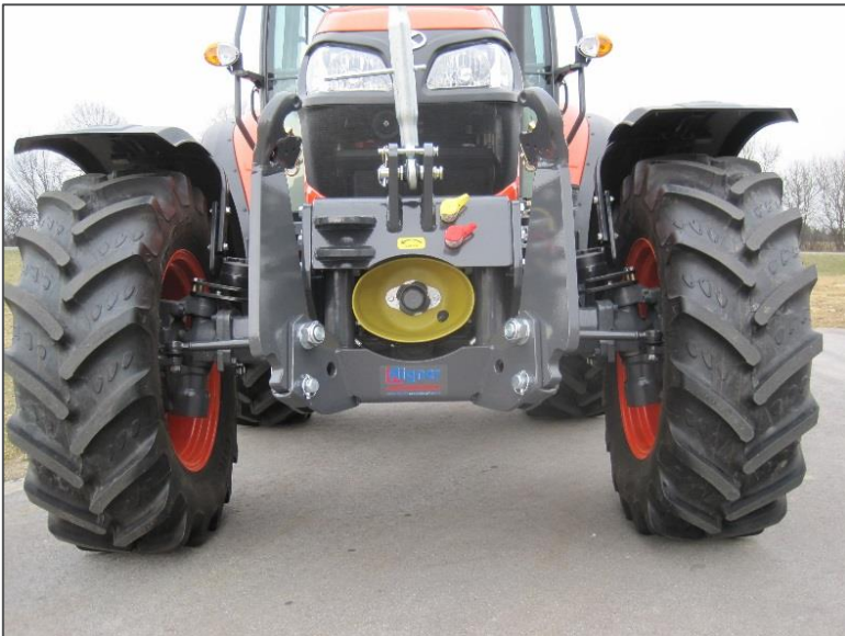
Lower links fold inward diagonally
