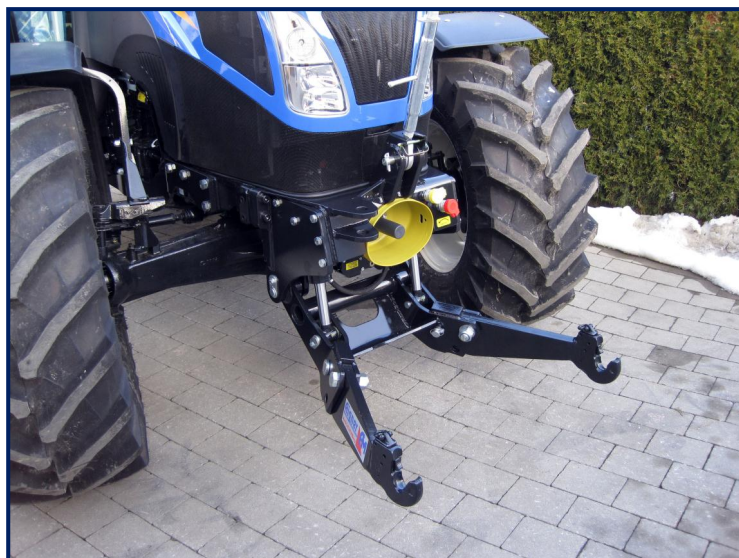
Front linkage and PTO are a compact unit
