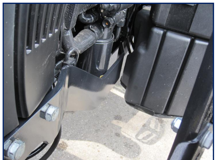
Stable frame up to clutch housing – uninhibited front axle oscillation
