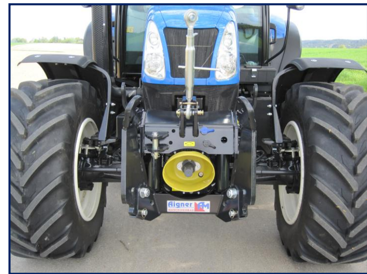
Lower links fold inward diagonally
