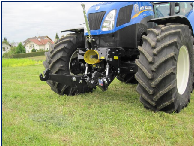
Steering angle and the front axle oscillation completely maintained!
