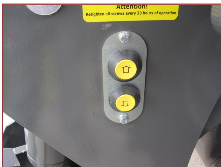
Front linkage remote control (only with electr. control unit)
