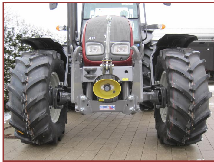
Lower links fold inward diagonally
