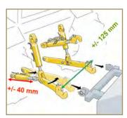
The Hydraulically adjustable stabilizer gives the opportunity to side shift the complete 3 point linkage including any implement laterally up to +/- 250mm.
